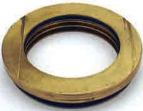
Failed Seal Resulting from Improper Installation
