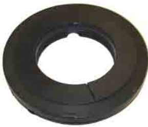
Failed Seal Resulting from Improper Fit
