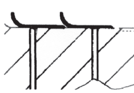
Two sleeves for double seal installation.
